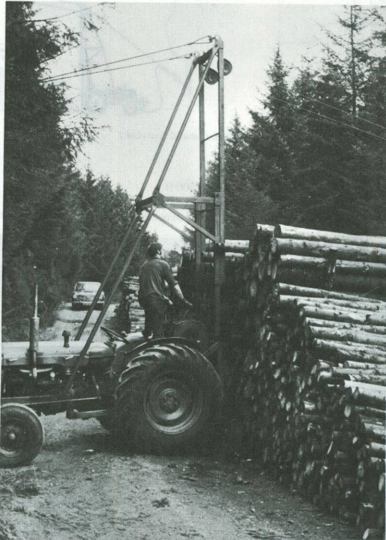
Model 4000/2 "Igland" double drum winch rigged for running skyline yarding of shortwood. (Courtesy James Jones & Sons, Ltd.)
