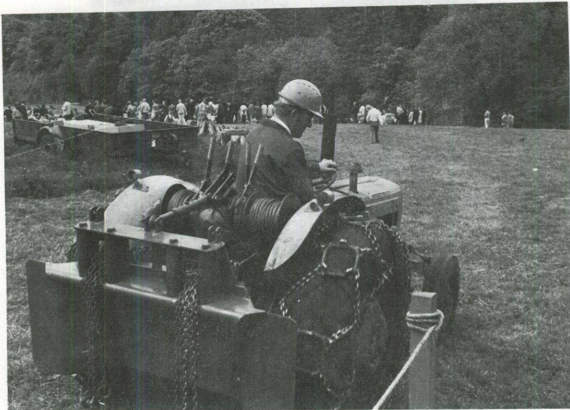
Model 3000/2 'Igland' double drum winch rigged for ground skidding.
